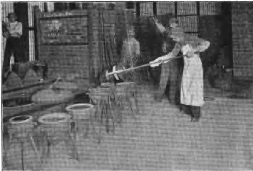
FIG. 67.—POURING THE BULLION : THE GREAT BOULDER PERSEVERANCE.
