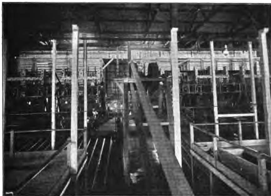
FIG. 46.—THE GOLDEN HORSE-SHOE 50-STAMP BATTERY (INTERIOR).
