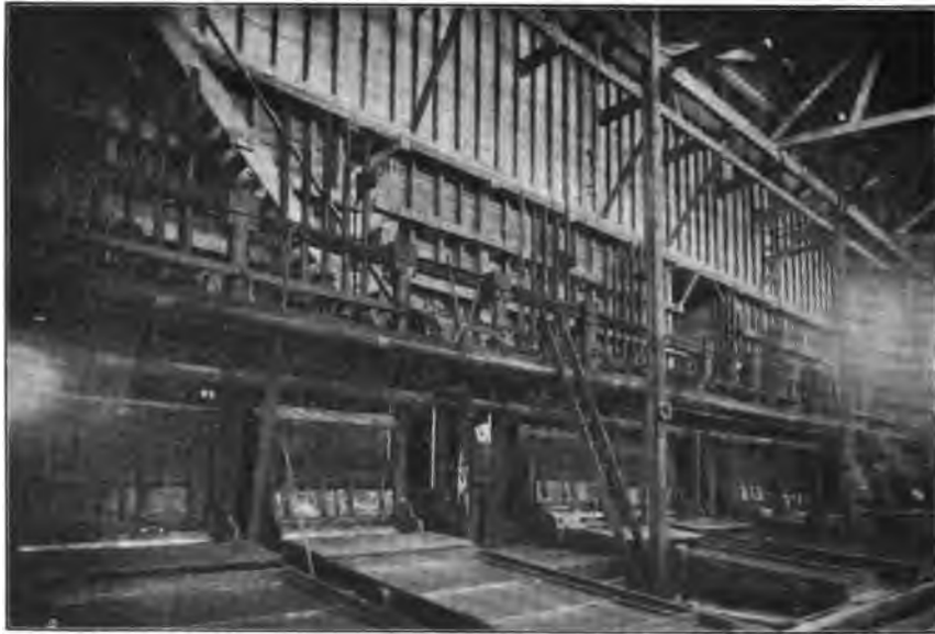
FIG. 64.—INTERIOR OF THE IVANHOE BATTERY. (Showing apron-plates and head of canvas tables.)
