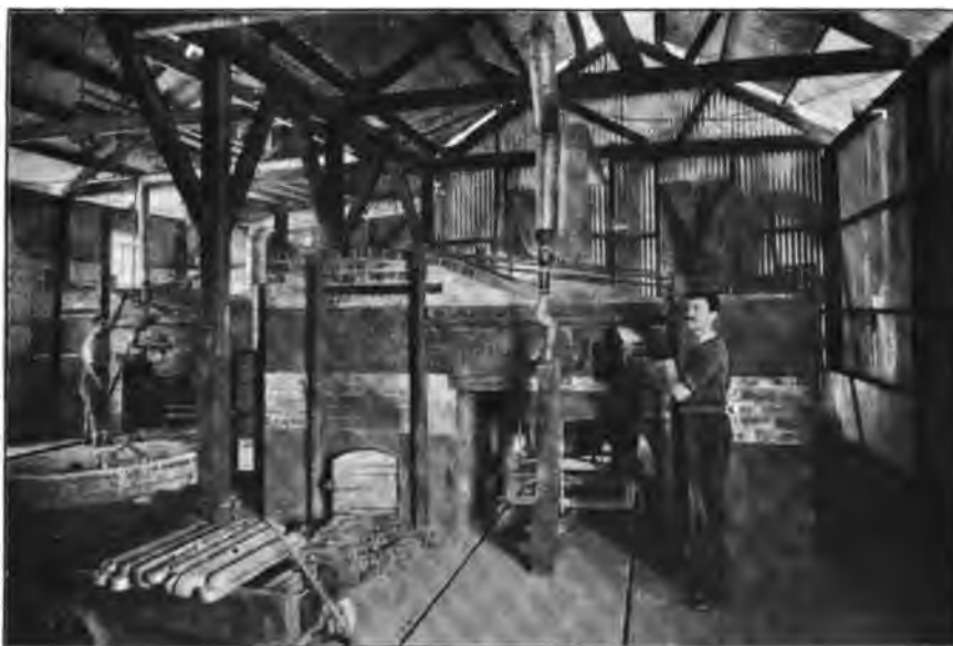
FIG. 66.—CUPELLATION FURNACES, GOLDEN HORSE-SHOE WORKS.
