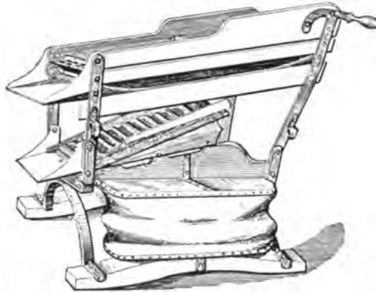
FIG. 6.—DRY-BLOWING MACHINE (LORDEN'S).
