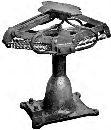
Fig. 258. OVERHEAD CONTACT DEVICE OF NEW YORK CENTRAL LOCOMOTIVE.
