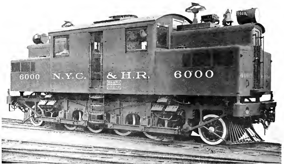
Fig. 253. ELECTRIC LOCOMOTIVE FOR NEW YORK CENTRAL RAILROAD. WEIGHT, 85 METRIC TONS.
