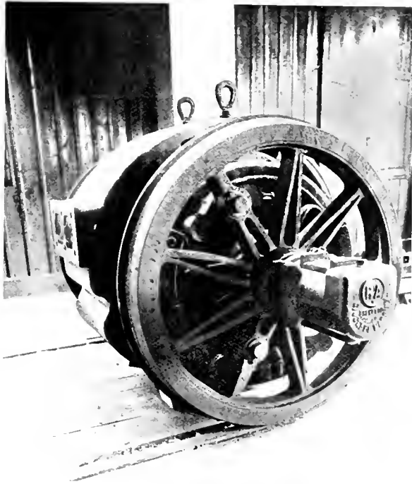
Fig. 304. THREE-PHASE MOTOR MOUNTED ON AXLE OF VALTELLINA MOTOR CARRIAGE.
