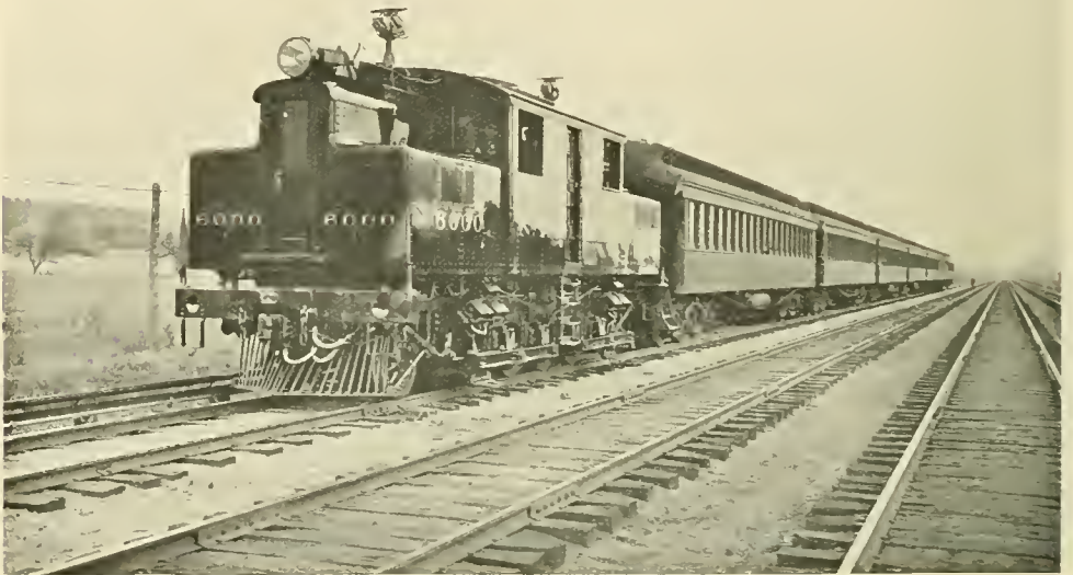
Fig. 262. NEW YORK CENTRAL LOCOMOTIVE HAULING A SIX-CAR TRAIN DURING ONE OF THE TESTS OF NOVEMBER, 1904.
