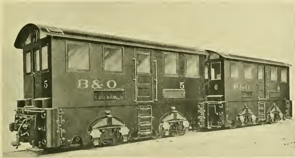
Fig. 270. BALTIMORE AND OHIO TWO-UNIT 1903 LOCOMOTIVE, WITH GEARED FOUR-POLE MOTORS. WEIGHT OF TWO-UNIT COMBINATION, 146 TONS.
