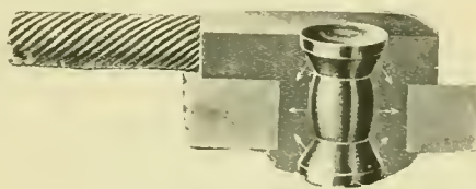
Fig. 237. GENERAL ELECTRIC Co. (U.S.A.) RAIL BOND: SECTION THROUGH BOND, SHOWING EFFECT OF COMPRESSION.
