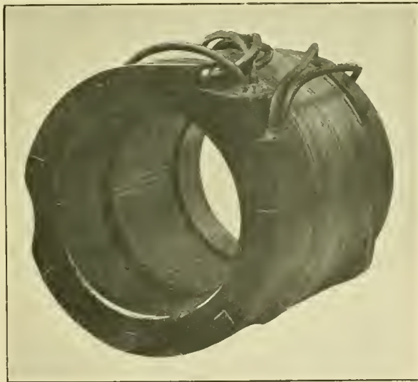
Fig. 365. FIELD FOR BRITISH THOMSON-HOUSTON Co.'s COMPENSATED SERIES SINGLE-PHASE RAILWAY MOTOR.
