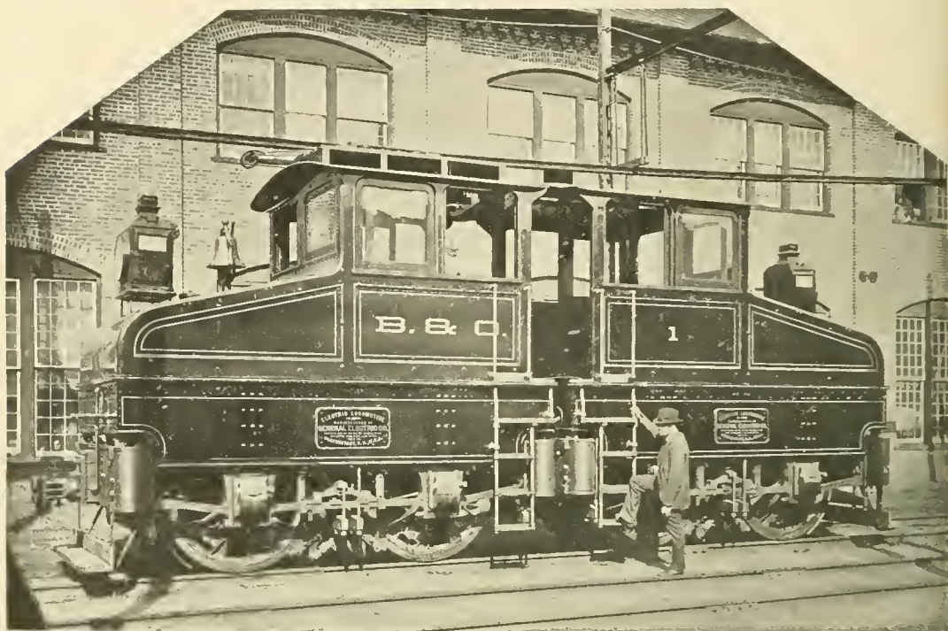
Fig. 268. BALTIMORE AND OHIO 1896 GEARLESS SIX-POLE LOCOMOTIVE. COMPLETE WEIGHT, 87 METRIC TONS.
