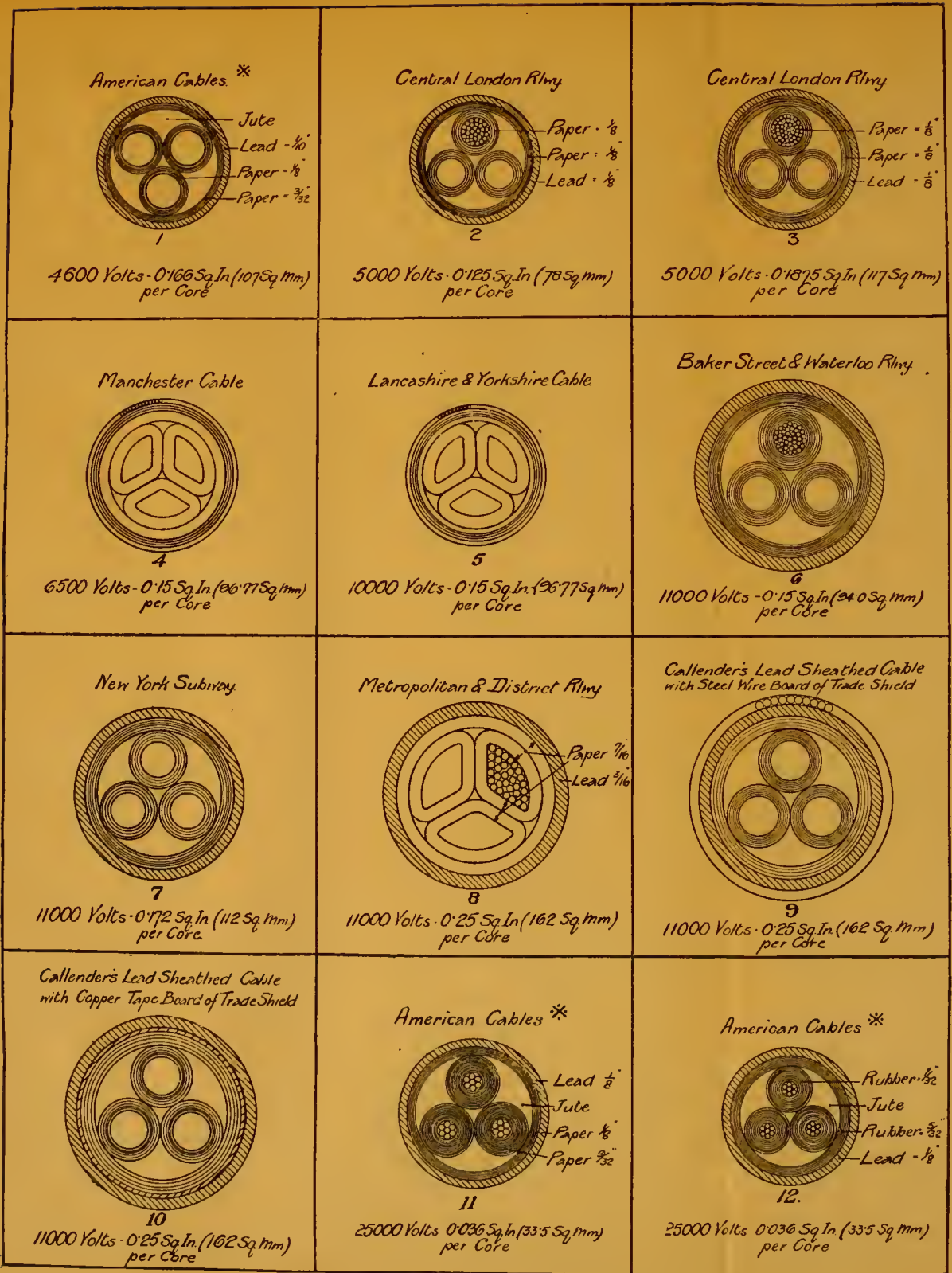
Fig. 143. SECTIONS OF VARIOUS HIGH TENSION CABLES.
