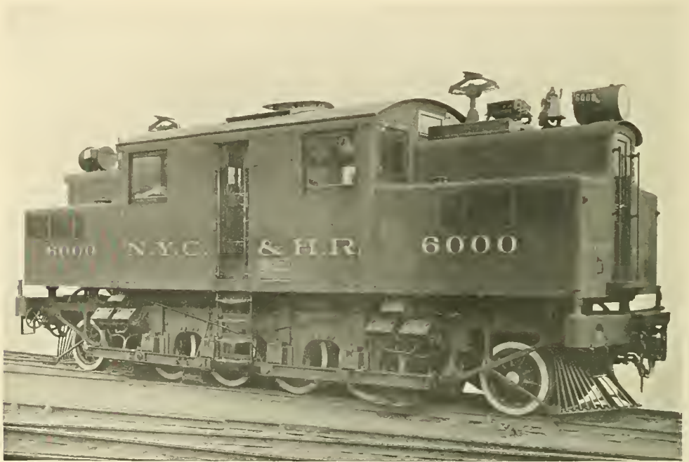
Fig. 253. ELECTRIC LOCOMOTIVE FOR NEW YORK CENTRAL RAILROAD. WEIGHT, 85 METRIC TONS.
